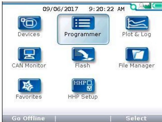
The Programmer\* app is where parameters, monitor variables, active-faults, and the fault -history are accessed. There are no separate monitor and diagnostics apps on the main screen. This chapter covers all of the items that can be accessed with the Programmer. It is recommended that the Device manual be consulted for explanations of the read/write and read only variables viewable within Programmer.
