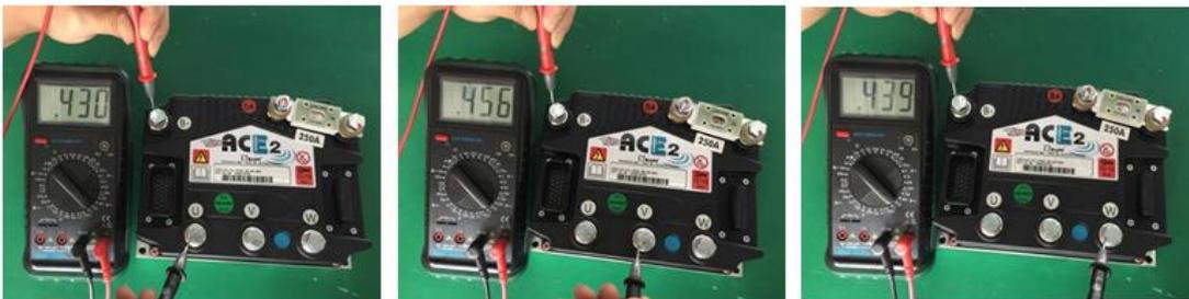
Test 2: measure the diode voltage to u, V and W with red lead, and B + with black lead.
