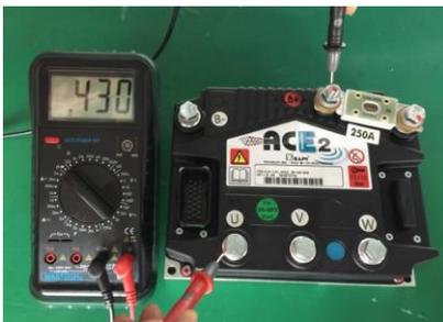
Note: The multimeter pointer cannot be reversed
