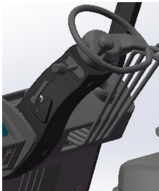
Figure 2-7 Steering control device
