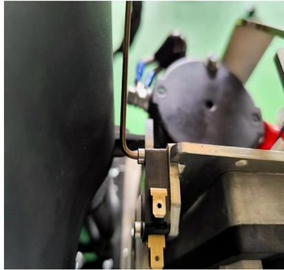
Remove the two fixing bolts of the limit switch with the 2.5mm hex socket and remove the limit switch
