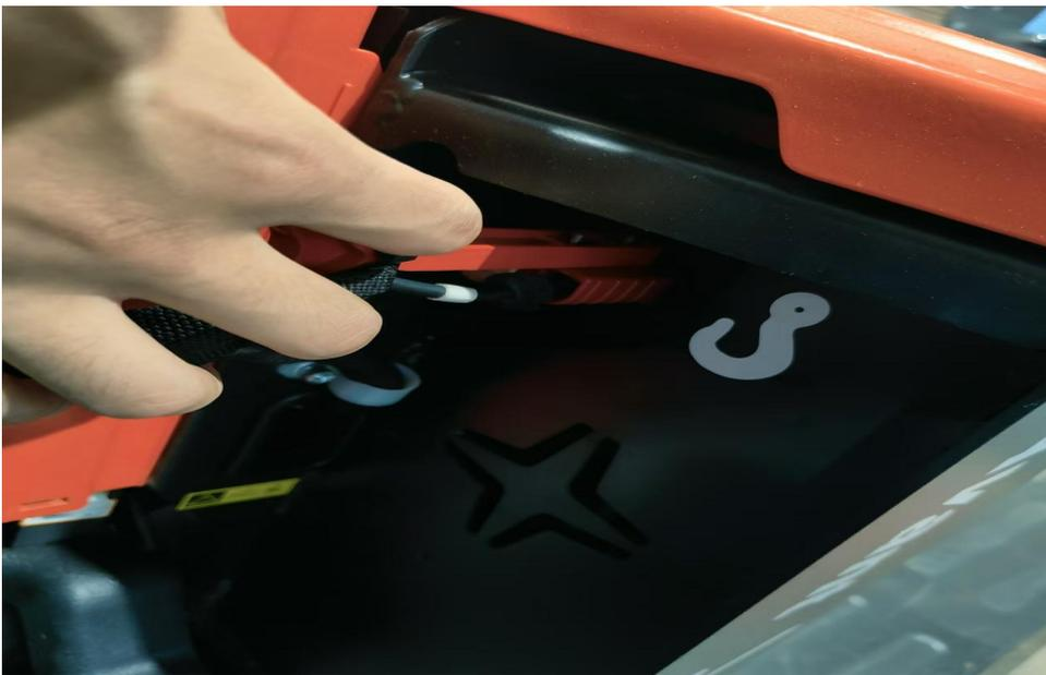
Grab the groove on the back and pull the battery up
