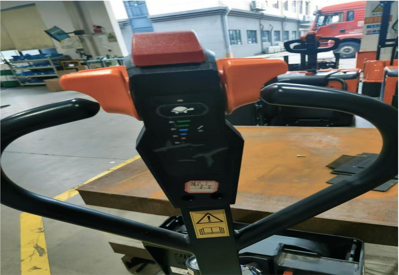
**Remove the connector to remove the handle front cover**
