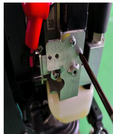
Remove the contactor by unscrewing the two fixing bolts with a Phillips screwdriver
