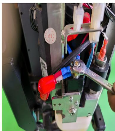
Remove the two nuts of the contactor pile head with a 10mm open end wrench
