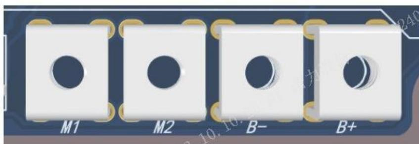
M1: motor+      M2: motor -      B-: battery -      B+: battery +
