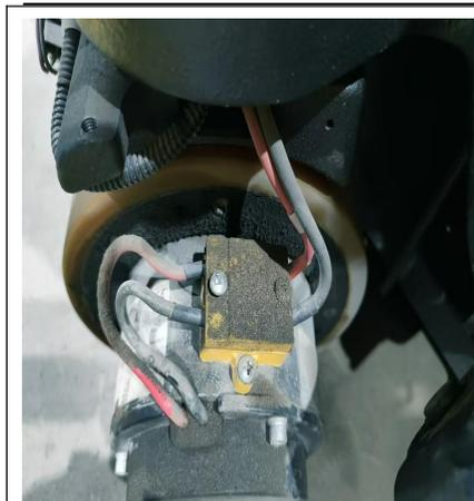
Open the junction box with a Phillips screwdriver and remove the nuts on the M1 and M2 terminals of the drive motor with a 10mm open end wrench
