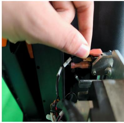
Remove the connector on the limit switch
