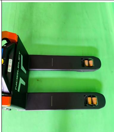
Power the vehicle and press the lowering button to drop the fork
