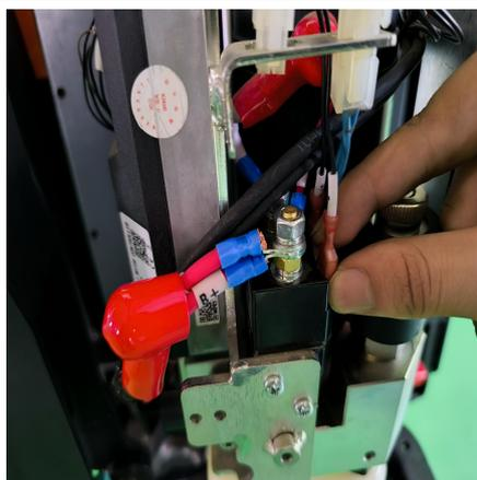
Remove the upper connector of the contactor
