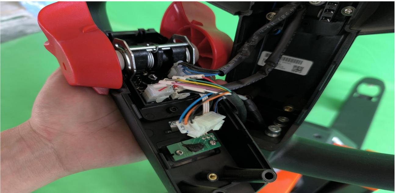
Remove the two bolts on the side of the rear cover of the handle using a 3mm hex key
