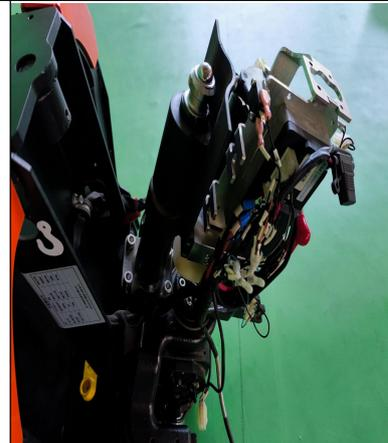
Gently lift the frame, and when the piston rod is off the upper seat, tilt the back half back to place it
