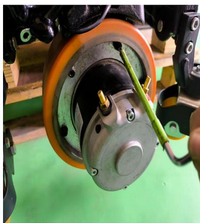
Use a 5mm hex socket to remove the six bolts fixing the drive wheel ring, that is, remove the wheel ring. Pay attention to the positioning holes and pins when installing the drive wheel ring
