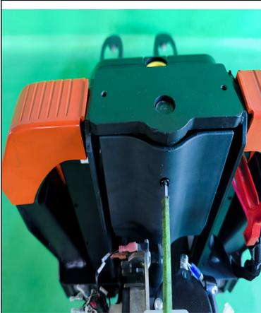
Remove the cylinder head positioning bolts using a 5mm hex wrench
