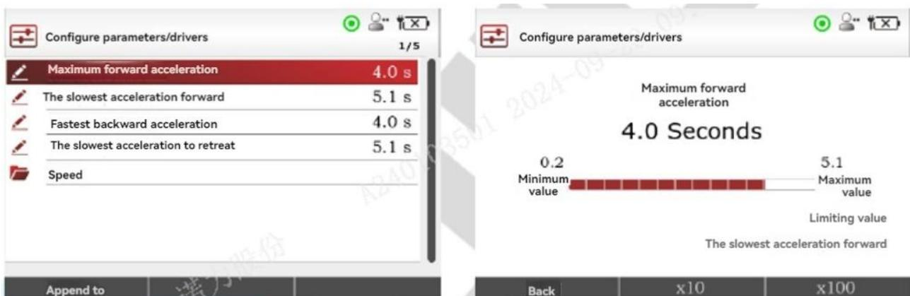
The configuration parameters are set in detail
