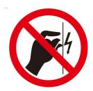
(1)Do not touch the positive and negative terminals of the battery with both hands at any time.
