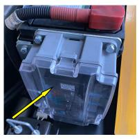
The fuse box is installed in the electrical box.
