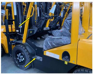
Safety pedals are equipped in both sides of the vehicle body. Safety handle is located on the left support of overhead guard. It is necessary to use safety pedals and safety handle when getting on or off the vehicle (Need to get on and off the truck from the left).
