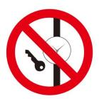
(3)Always wear insulated gloves when operating and maintaining the battery system, and do not wear metal jewelry such as watches.
