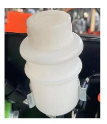
The brake fluid reservoir is installed in the left side of inner surface of the instrument panel. The reservoir is semi-transparent so that we can observe the level of the brake fluid from the outside.
