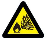
(4)Keep the battery system away from highly corrosive and flammable environments and away from sources of ignition when in operation.
