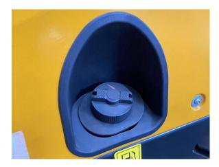
Fuel tank cap is located on the left rear side of the vehicle body. To open it, just turn it in counterclockwise direction.
