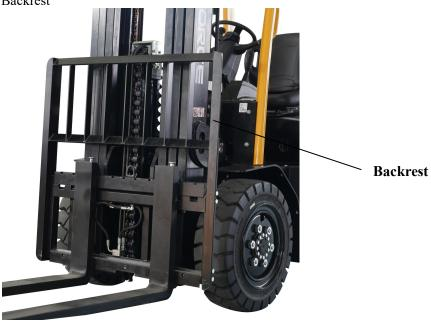
Examine whether or not the mounted bolts for backrest are loosened, and they shall be tightened up when required.
