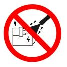
(2) While cleaning the vehicle, prevent high-voltage components from contact with water to avoid adverse consequences.
