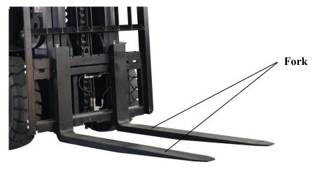
Examine the mounting status of for positioning pin, and whether or not the fork is distorted or cracked.
