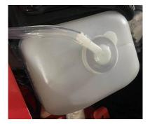
Check the liquid level of the coolant recovery tank. The liquid level should be in a place between lower and upper scale marks. Add coolant if necessary.
