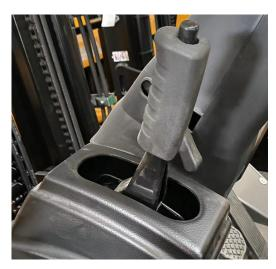
In parking brake, this handle acts on the front wheel through back tip, for brake to generate braking force. Push forward the handle to loosen the brake.
