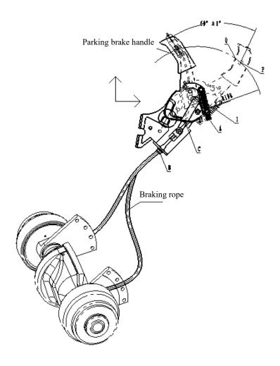
Fig 7-7 Parking Brake Device
