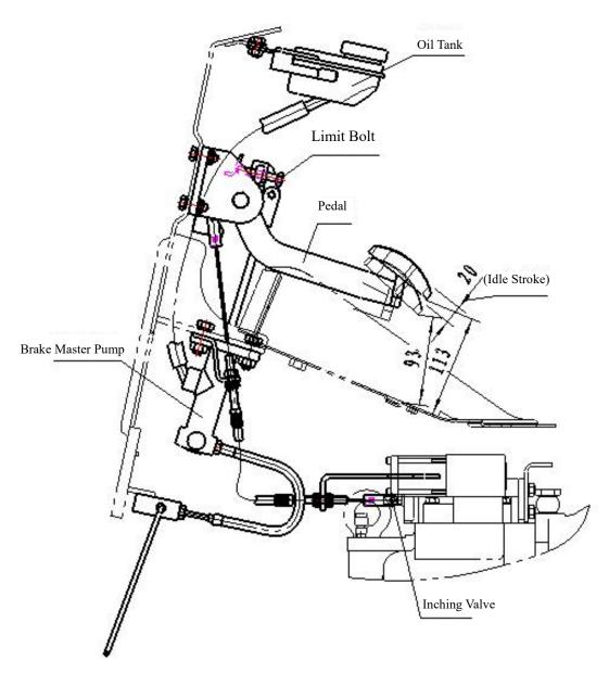
Fig 7-8 Adjustment of Brake Pedal
