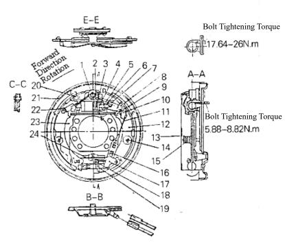
Fig 7-4 3t and 4t Wheel Brakes
