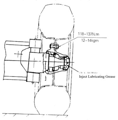
Fig 6-2 Adjustment for Pre-tightened Load
