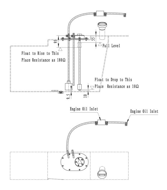
Fig 1-4 Fuel Tank (Gasoline Forklift Truck)
