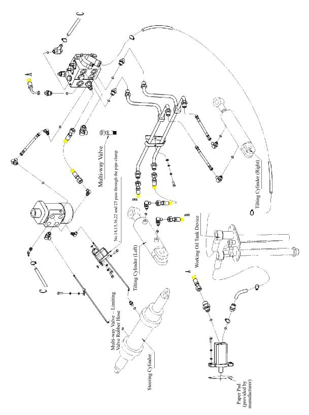
Fig 9-20 Schematic Drawing of Hydraulic Pipeline (Diesel and Gasoline Forklift Trucks)
