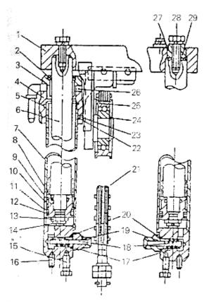
Fig 9-8 Lifting Cylinder
