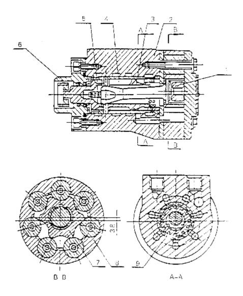
Fig 5-2 Cycloid Fully Hydraulic Steering Gear
