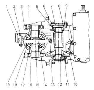
Fig 2-12 Speed Reducer and Speed Differential
