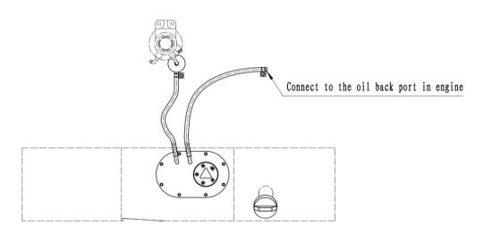
Fig 1-3 Fuel Tank (Diesel Forklift Truck)
