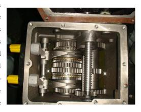
Fig. 2-2 Gear-Shift Mechanism
