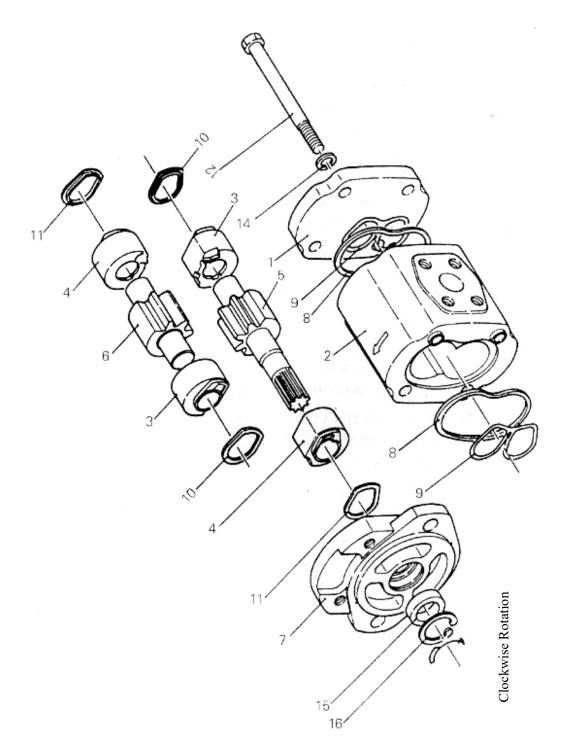
End Cover 2. Pump Body 3. Bearing 4. Bearing 5. Driving Gear 6. Driven Gear 7. Front End Cover 8. Seal Ring 9. Seal Ring 10. Seal Ring 11. Seal Ring 12 Bolt 13. Lock Washer 14. Oil Seal 15. Locking Collar
