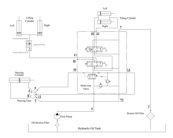
Fig 9-7 Oil Circuit of Hydraulic System
