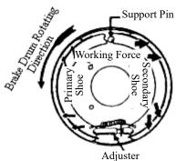
Fig 7-5 Brake Actions during Forward Running Process
