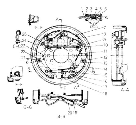
Fig 7-2 1-1.8t Wheel Brake (Left)
