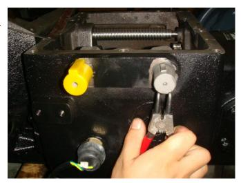
(7) Gently knock at the head of rotary rod (Attention: Not to be heavily opened), and taken off the rotary rod (Fig 2-19).
