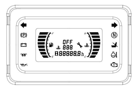
Note: the hourmeter and weighing meter share a digital display zone; when it is powered on, it displays the hour counter and funnel chart; press any key, and it displays the weight value and "kg" and at the same time, the hourmeter funnel chart is off.
