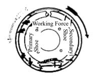
Fig 7-6 Brake Actions during Reversing Process
