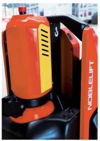
For the pallet trucks there are no hoses or pipes used in the hydraulic lifting circuit which significantly improves reliability and reduces the amount of potential problems related to leakages through connectors or their seals.
