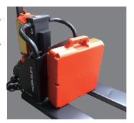
The PTE 20B truck is equipped with maintenance-free AGM battery pack, the charging time is 8 hours.
