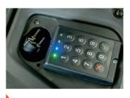
The option of PIN-code panel access, which works not only with PIN-code but also with access cards (RFID), can significantly simplify the procedure of access limitation for the fleet which may be used by more than one operator.
