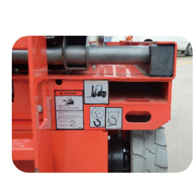
Standard transportation forklift holes and crane holes
