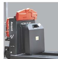
The steel battery cover can be easily opened allowing quick battery replacement.
