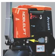
An external programming port makes parameter adjustments and overall vehicle maintenance more convenient and efficient.
