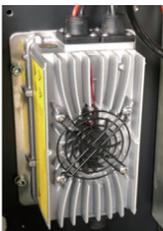
The charger with current 12A is used. The standard charging time is 7 hours
