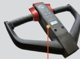
Tiller is made of fiber glass material for high strength.
